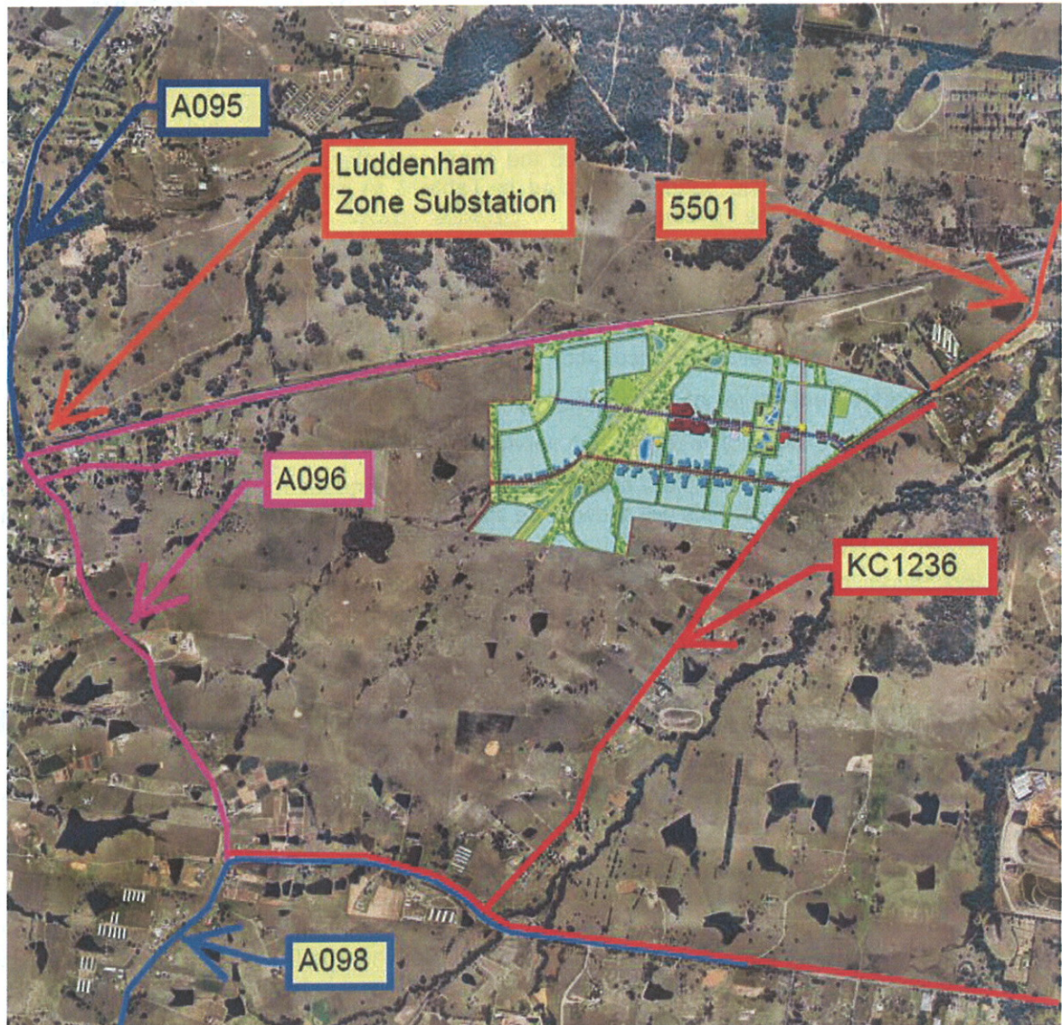
Plate 5 Overhead High Voltage Lines
